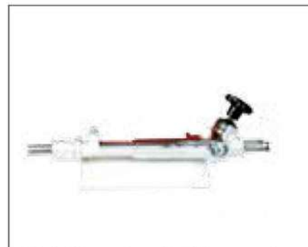
■ Variable rack and pinion steering anatomical model
